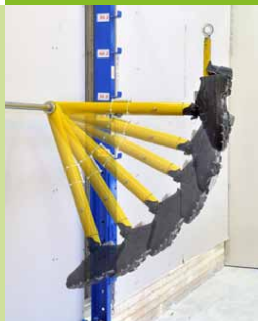
Figur 2: Hard Body Impact, Gyproc modificeret, ISO 7892 part 2 1998 30 N m
